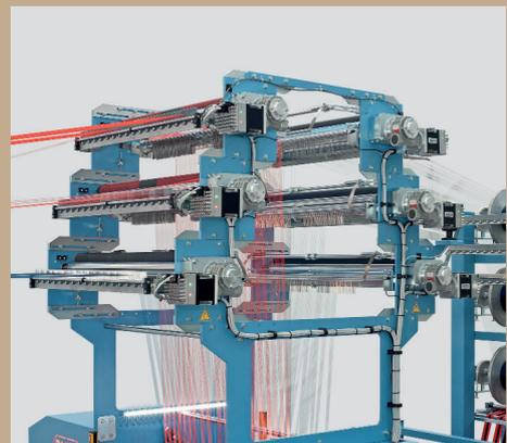
Special configuration with 6 electronic control feeders (on request)
