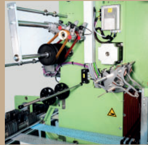
Heald frame and harness drive with electronically controlled weft and binder transport
