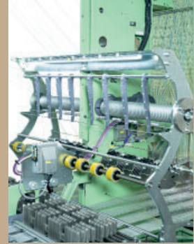
Electronically controlled feeding for weft, catch and rep thread
