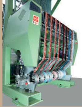
Electronically controlled winding up
