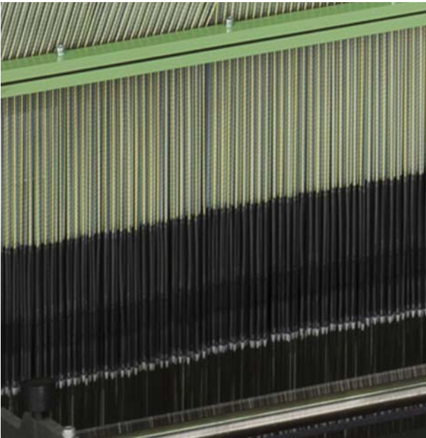
Delta harness link: patented plastic link, which can be reopened
