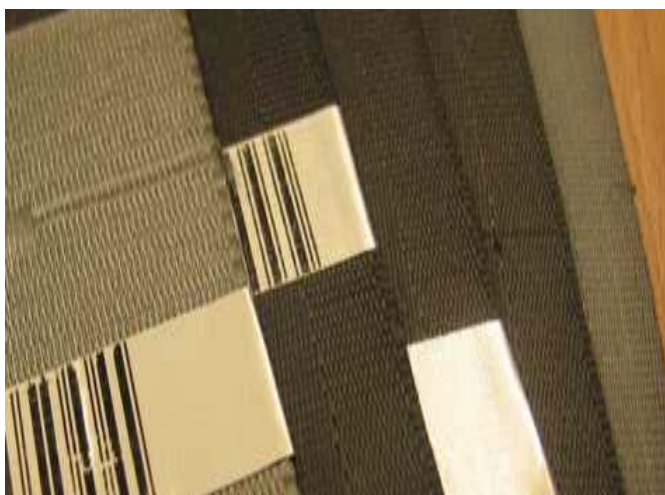
Tape faults marked with barcode labels
