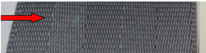
Dirt / Dye spots, stains of grease, oil, chemicals
