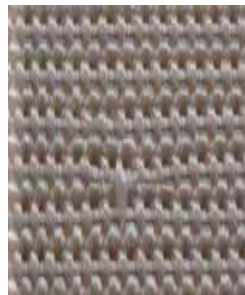
Dirt / Dye spots , stains of grease, oil, chemicals, pattern faults
