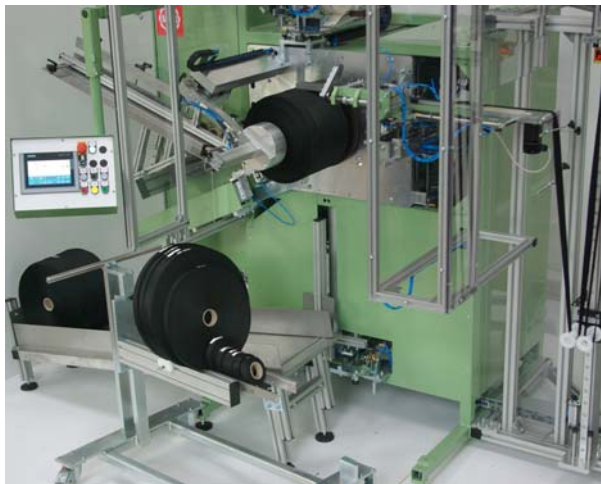
UV60-RS with roll-off shaft for spools resp. magazine wagon for rolls
