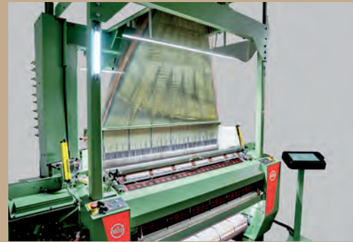
Light barrier and MLC touch panel
