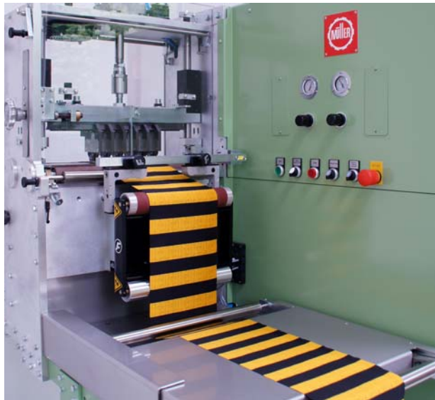
Supply of label ribbon from roll
