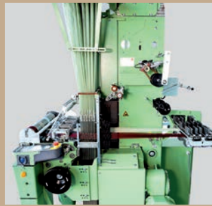
Heald frame and harness drive with electronically controlled weft and binder transport
