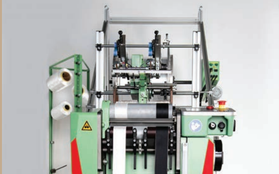
NG3.1 28G with electronically controlled take-off.
