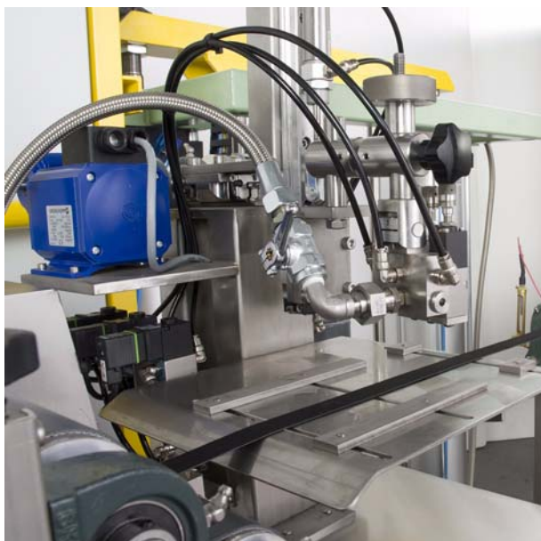
Feed side and coating unit
