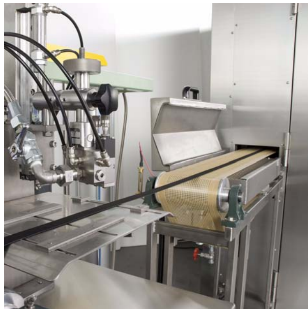
Horizontal tape drying behind the short steamer
