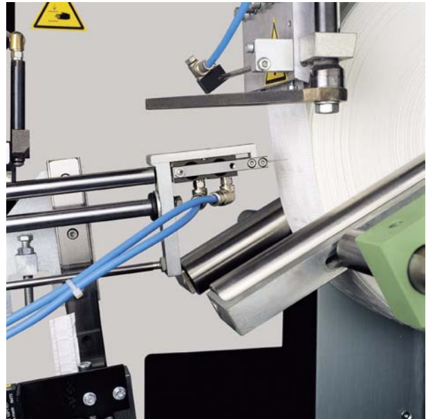
RAM-500 option: needle device for tape end fixing
