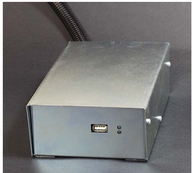
External UNI-NETWORK interface for UNI controls
