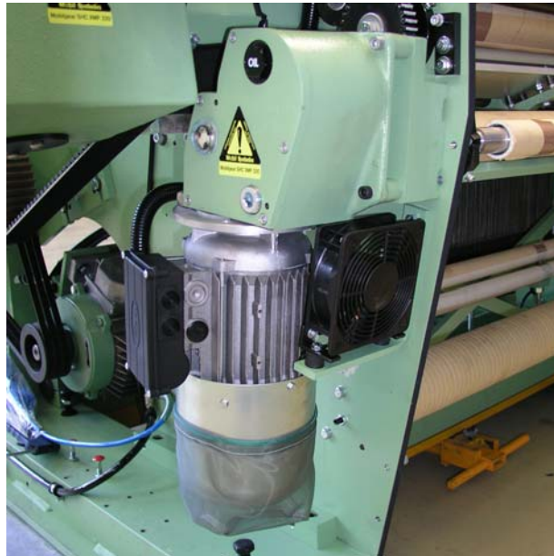
VARIPICK – frequency converter controlled, 3-phase motor
