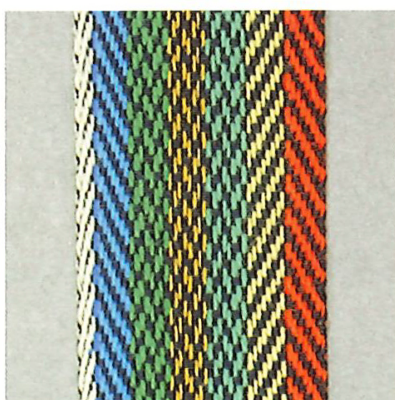
Figure 264: 4-end broken twill (variation on uniform line twill) K\frac{2}{2}X
