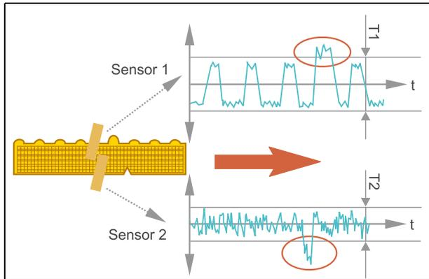
The diagram shows that signals from two sensors are used to check the tape
