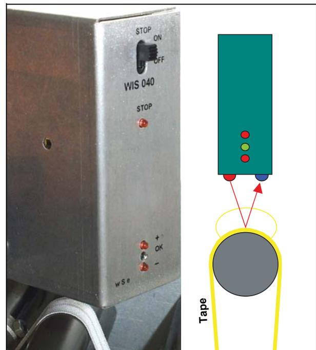
Inspection sensor, picture and schematic diagram
