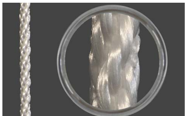
Non-elastic rope sample, uni Ø 3.5 mm
