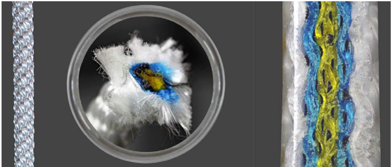
Core-sheath rope with a diameter of 11 mm, external structure (left), core-sheath close-up (centre), internal structure (right)
